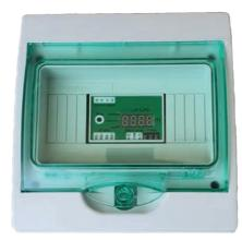
Leak Detection System uses Locating Panel (C-LP) as a Sensor Interface Module (SIM) to detect the liquid leak and communicates to BMS System. The alarms, faults and power LEDS display the current system status while the built-in distance locating feature can identify where the leaks occurs.
